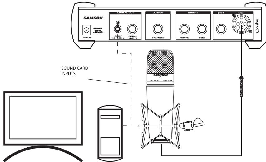
The C valve's A-to-D converter has a selectable sampling rate. Simply put, the sampling rate is how many times per second the A-to-D converter takes a digital picture of the sound. Use the 48 / 96 switch to select the sample rate that is compatible with your digital recording device.
