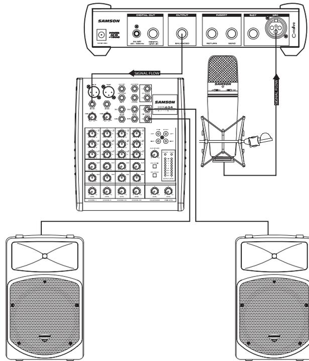
In this example, a condenser microphone is connected to the C valve's MIC input using a standard XLR cable. To make a balanced connection, the C valve's output is connected to the input of a standard PA mixer using a standard 1/4-inch TRS (TIP-RING-SLEEVE) cable. The mixers main left and right outputs are connected to powered PA speakers (for example, the Samson dB500a).
