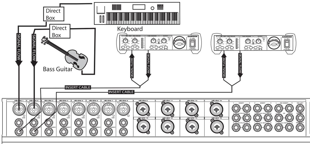
You can use the C valve to “warm-up” the signal from recorded tracks or instruments such as digital electric piano or bass, to name a couple. The example above shows the two C valves inserted into the insert point of a mixer on the keyboard and bass channels. Set the input and output level so that you get unity gain (the same level in and out), and then use the SATURATION control to adjust the amount of tube sound.
