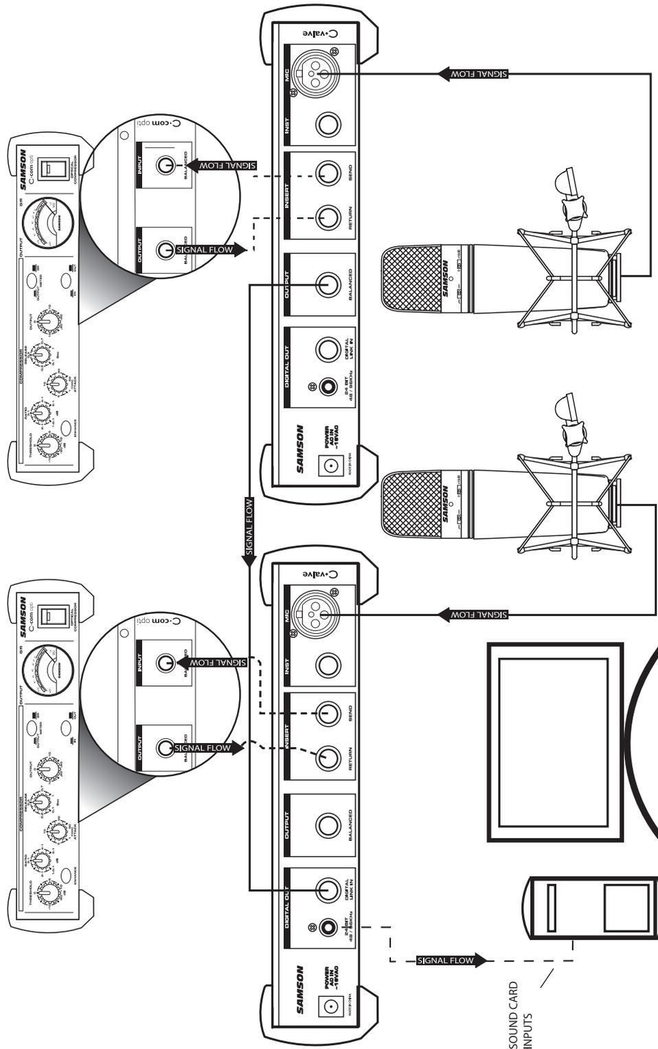
*In this example, two C valves are used for recording a stereo signal to a computer based hard disk recorder. The balanced OUTPUT of the second C valve is connected to the DIGITAL LINK input on the first C valve so that both signals are sent the S/PDIF out on C valve one. For extra dynamics control, a compressor (in this case the Samson C com opti optical compressor) is connected to each C valve via the INSERT SEND and RETURN jacks.*
